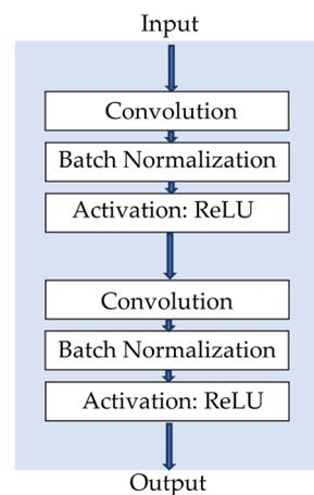
**Figure 3.** Convolution block.
