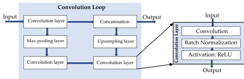
**Figure 4.** Convolution loop.
